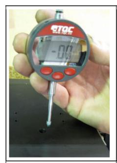
Insert the micrometer in the designated hole on top of the TQC Manual Cupping Test.
