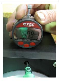
Keep the micro meter secure and straight and fix the micrometer by using a 1mm Allen key.
